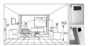
Receivers - Install away from conductive elements, metal surfaces, electrical cables or excessive heat.
