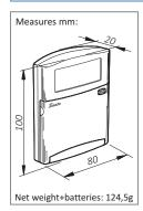
Power supply:. 2 alkaline battery 1,5V LR03 (AAA) Low battery indicator:..... Regulation scale:..... from 5 to 35°C Transmission frequency:...... 868,3 MHz Ambient temperature:..... from 0°C to 40°C Storage temperature:..... maximum 50°C % Relativity Humidity operating:.. from 20 to 85% Dregee of protection:..... IP20 Action Type According EN 60730:..... 1.B Homologated:..... CE Approximate maximum distance between emitter and receiver:...... 130m in free field
