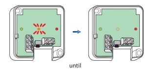
If you have installed the batteries, before coding it, you have to remove them & wait until the display shut down
