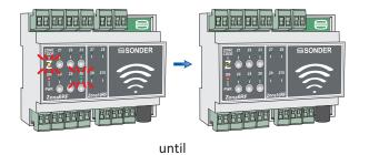
If you have installed the batteries, before coding it, you have to remove them & wait until the display shut down
