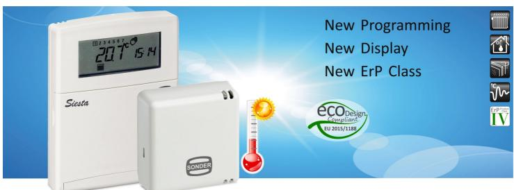
Daily and weekly chronothermostat for heating only, allows programming by blocks, complies with ErP class IV (2%), can be selected all/nothing or modulating action in time. It also incorporates shutdown in case of window opening detection. Battery-powered wire connection.
