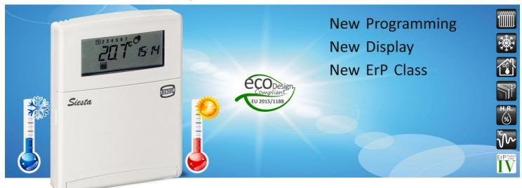
Daily and weekly chronothermostat for Heating / Cooling, allows programming by blocks, complies with ErP class IV (2%), can be selected all/nothing or modulating action in time. It also incorporates shutdown in case of window opening detection. Wired and battery powered.
