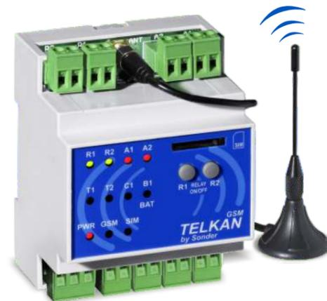
Remote control via GSM that works by sending and receiving SMS (configurable in 2 languages, Spanish / English). Ability to operate powered 12V ideal photovoltaic installations.
